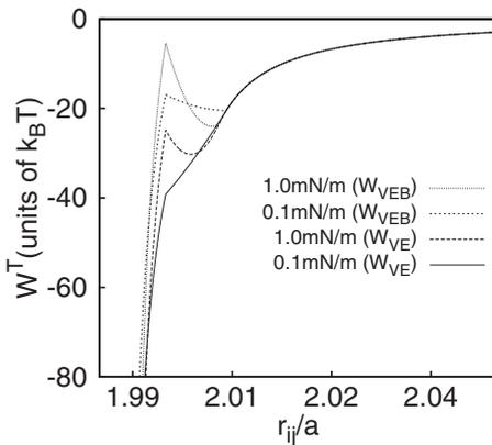
FIG. 15. Interaction potential between two droplets of 1  $\mu\text{m}$  for two different interfacial tensions. Lower curves correspond to absence of bending energy.
