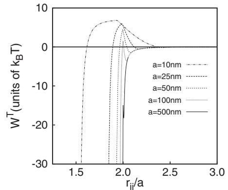
FIG. 9. Interaction potential for two deformable droplets of equal size. The interfacial tension is 1 mN/m. Droplet radius from 10 to 500 nm.
