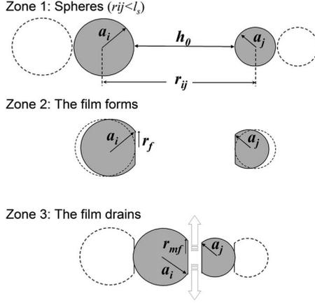
FIG. 4. Definition of  $h$  and  $r_f$  depending on the separation  $r_{ij}$  used in order to introduce them in equations for  $W$  and  $D$ , following the three-stages deformation process model. Distances and droplet deformation were exaggerated for a better visualization.
