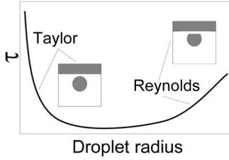
FIG. 1. Schematic illustration of the variation of the critical time vs. droplet radius obtained experimentally by Basheva *et al.* [35] for a system of one droplet coalescing with a planar liquid interface by effect of the buoyancy force. Two regimes are observed: the one of small droplets behaving as spheres (micron-sized droplets) and the one of larger droplets behaving as planar disks (millimetric-sized droplets).
