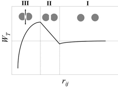
FIG. 3. Interaction potential between two deformable droplets according to the three-stages collision model: (i) the droplets keep spherical until reaching a surface-to-surface distance  $h_0$ . (ii) the film starts to grow at constant separation thickness. (iii) The film reaches the maximum radius and starts to drain.
