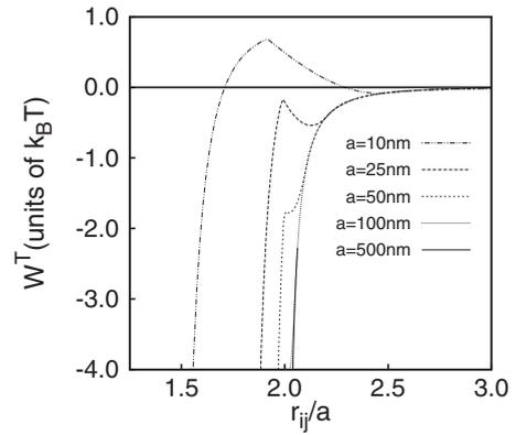
FIG. 8. Interaction potential for two deformable droplets of equal size. The interfacial tension is 0.1 mN/m.
