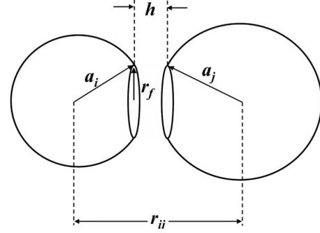
FIG. 2. Truncated spheres model for two deformed droplets of different radii  $a_i$  and  $a_j$ .
