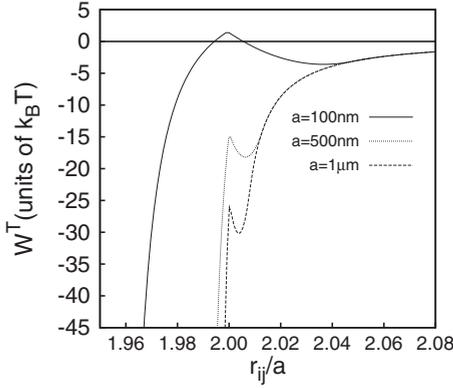
FIG. 10. Interaction potential for two deformable droplets of equal size. The interfacial tension is 1 mN/m. Droplet radius from 100 nm to 1  $\mu$ m.
