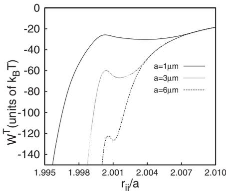
FIG. 11. Interaction potential for two deformable droplets of equal size. The interfacial tension is 1 mN/m. Droplet radius from 1 to 6  $\mu$ m.
