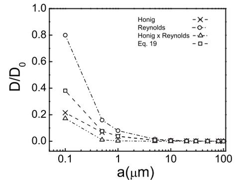
FIG. 5. Dependence of the different diffusion corrections on the size of droplet calculated according to Eqs. (19)–(21) and the Honig *et al.* correction ( $D = D_0 / \beta$ ). The values  $D/D_0$  were calculated by using the maximum film deformation  $r_{mf} = \sqrt{ah_0}$ . Lines are a guide for the eyes.
